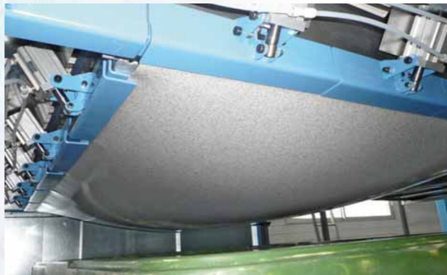
Sheet heating process Chauffe de la plaque
