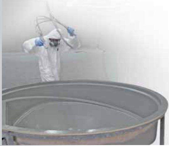
Gelcoat spray-up units Projection de gelcoat
