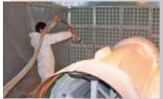
Gelcoat spray-up station Projection de gelcoat
